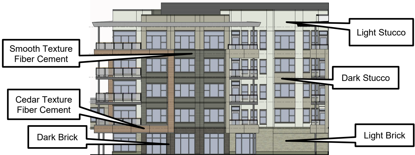
Figure 5. Building RB1.1 North Elevation Materials Detail
